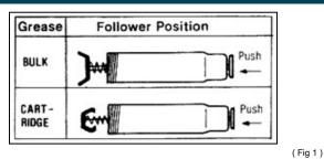
Installing Grease Cartridge
