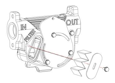
(Correct vane and rotor orientation)
